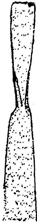
Figure 54. Framing Chisel PR87 545.6
