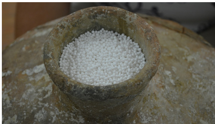
Figure 2: Volumetric measurement of a Canaanite jar filled to the narrowest area of the neck. Photo courtesy of the Uluburun Shipwreck Project.
